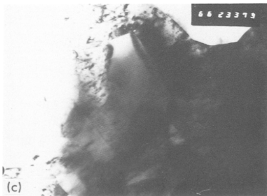
Figure 8 Electron micrographs of mullite-zirconia composites containing various amounts zirconia heat treated at 1300°C. (a) Pure mullite; (b) 0.5 wt % ZrO 2 ; (c) 5 wt % ZrO 2 .
